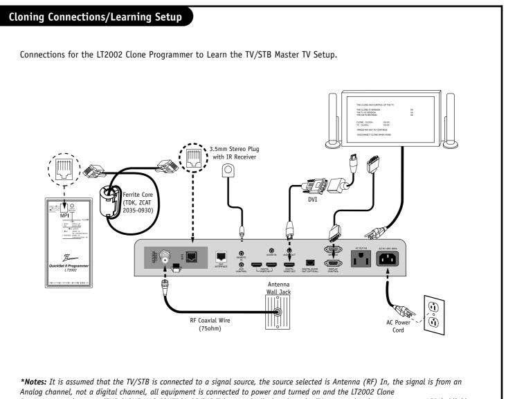
Programmer main menu (THE CLONE HAS CONTROL OF THE TV) menu is displayed on the TV screen, the clone programmer LED is blinking the required heart beat pattern, see above and next page.
